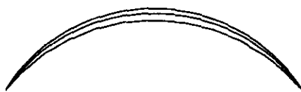
FIG. 16. Comparison of bubble size and shape at ncyc = 5000: Fine resolution grid—top shape; Medium resolution grid—middle shape; Coarse resolution grid—bottom shape.
